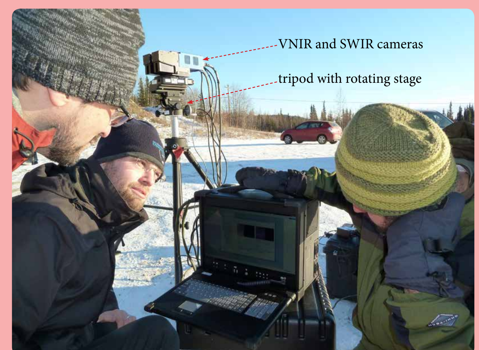
Use of the HySpex for mineral exploration near Murphy Dome.
